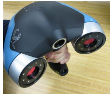
Figure 1. Creaform VIUscan device for optical shape capture ( www.creaform3d.com ). It acquires a surface mesh with positional accuracies up to 50 \mu\text{m} .
